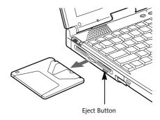
Figure 4-4 Loading/Ejecting a SuperDisk or 3.5" Floppy Disk
